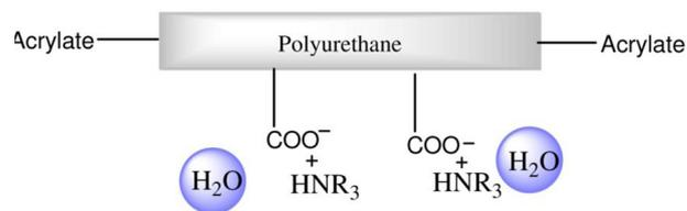
Stability of the WR-UAs strongly depends on the amount of water added to the neutralized UA oligomer. We observed two modes of stability failure:
