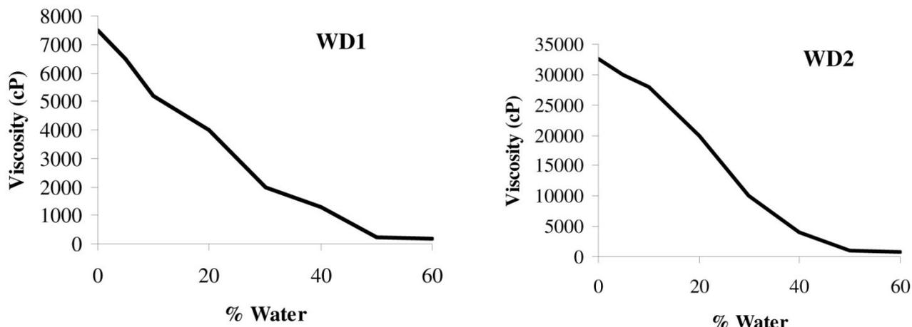
Two water dilutable oligomers are prepared: WD1 and WD2. Viscosity changes with the water dilution of these oligomers are given in Figure 5. Initial viscosities of the oligomers are much lower than WR-UAs and there is no sudden drop in viscosity with the water dilution.
